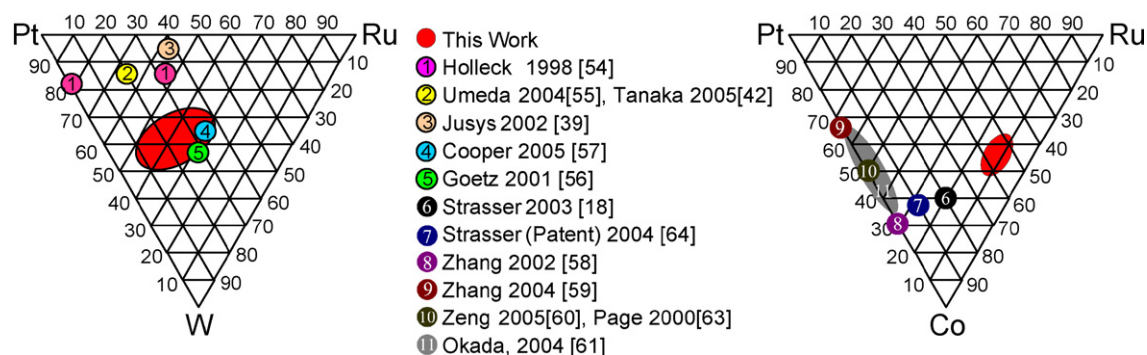
Fig. 10. Regions of the Pt-Ru-W and Pt-Ru-Co phase field that are active in the oxidation of methanol as reported by various groups.
